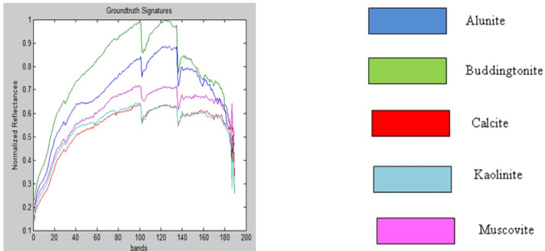
Fig 2. The groundtruth spectral signatures of five minerals
